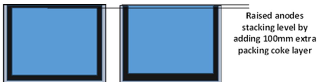
Figure 3. Difference in packing followed for the experiment with 1580 mm anodes.
