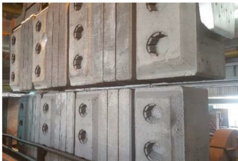
Figure 4. Clearance between the anode packets placed on central conveyor line (One packet is in lifted position).
